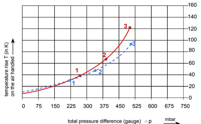
The performance curves are based on air at a temperature of 15 °C and atmospheric pressure of 1013 mbar with a tolerance of +/- 10 %. The total pressure differences are valid for suction and ambient temperatures up to 25 °C. For other conditions please confer with us.
