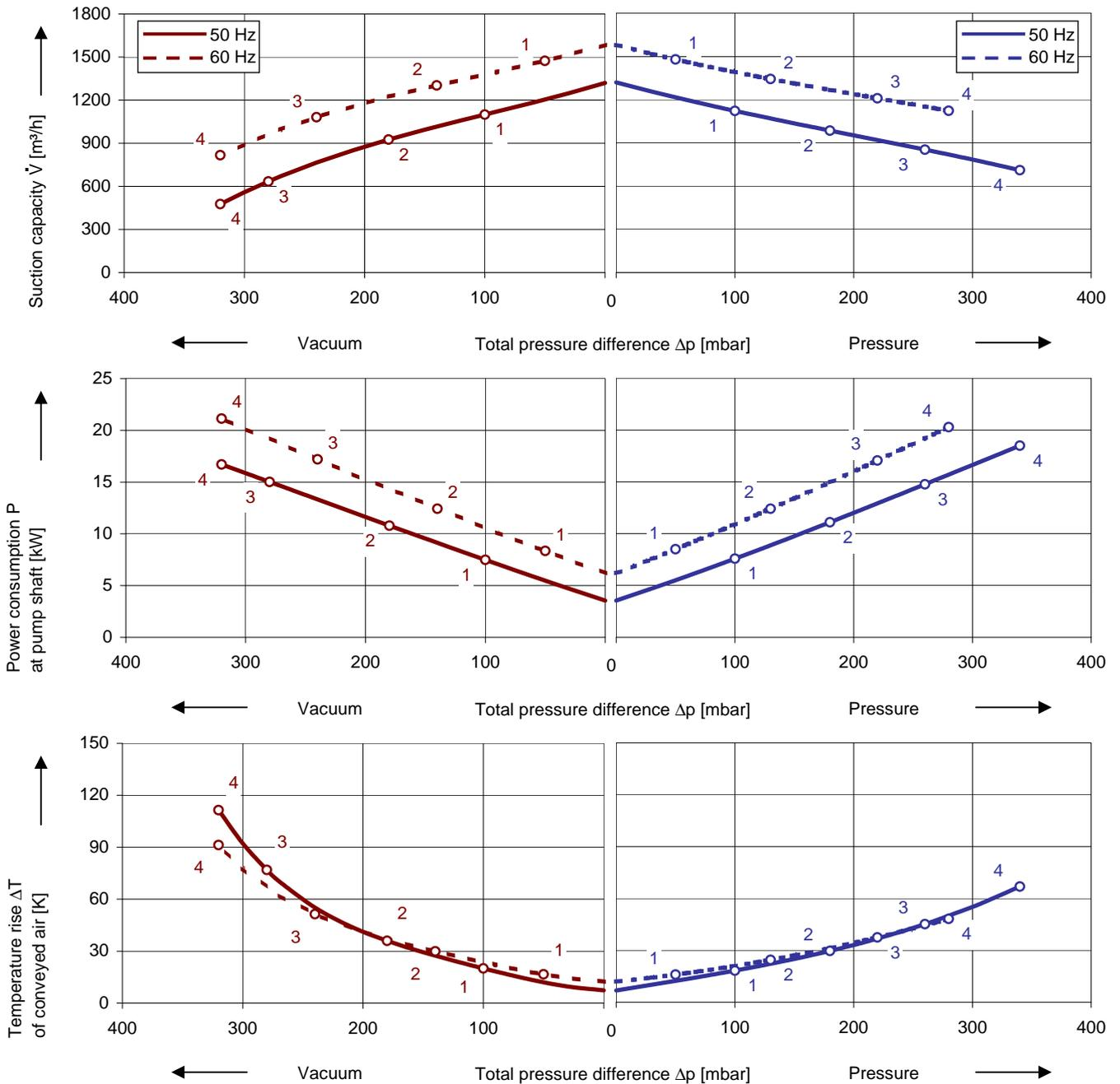
The performance curves are based on air at a temperature of 15 °C and an atmospheric pressure of 1013 mbar with a tolerance of ± 10 %. The total pressure differences are valid for suction and ambient temperature up to 25 °C. For other conditions please get in touch with us.
