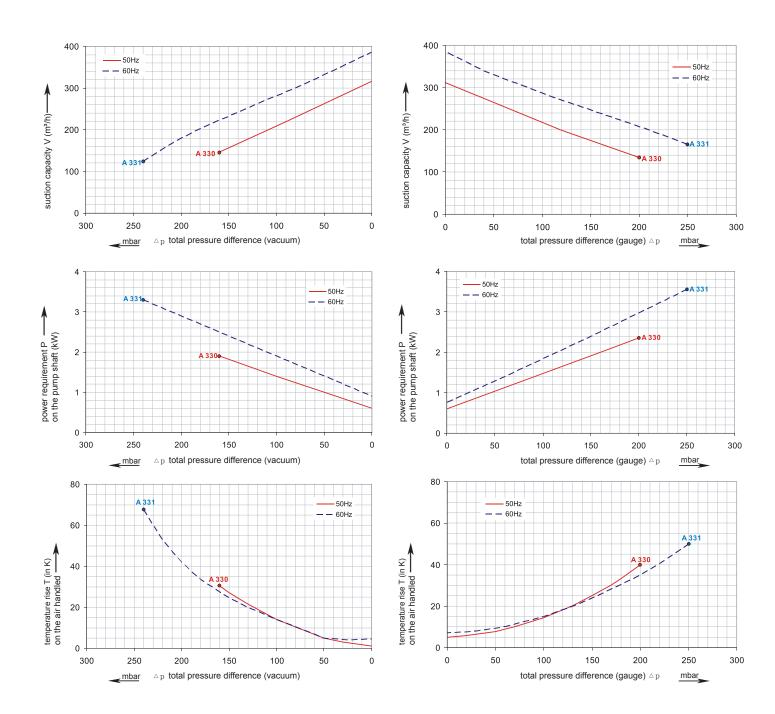
The performance curves are based on air at a temperature of 15  $^{\circ}$ C and an atmospheric pressure of 1013 mbar with a tolerance of +/- 10 %. The total pressure differences are valid for suction and ambient temperatures up to 25  $^{\circ}$ C
