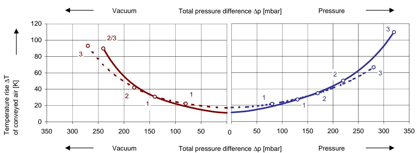
The performance curves are based on air at a temperature of 15 °C and an atmospheric pressure of 1013 mbar with a tolerance of  $\pm 10\%$ . The total pressure differences are valid for suction and ambient temperature up to 25 °C. For other conditions please get in touch with us.
