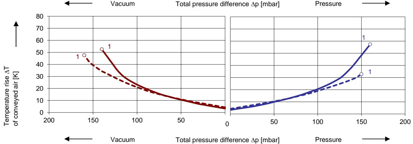
The performance curves are based on air at a temperature of 15 °C and an atmospheric pressure of 1013 mbar with a tolerance of  $\pm 10\%$ . The total pressure differences are valid for suction and ambient temperature up to 25 °C. For other conditions please get in touch with us.
